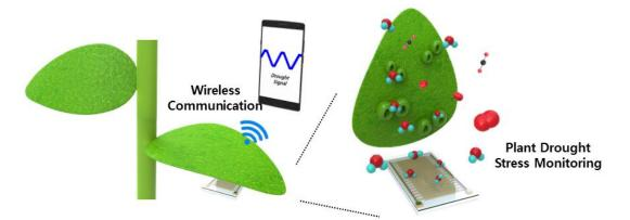
Figure 1. Scheme of the flexible PI-based plant drought stress monitoring system.
