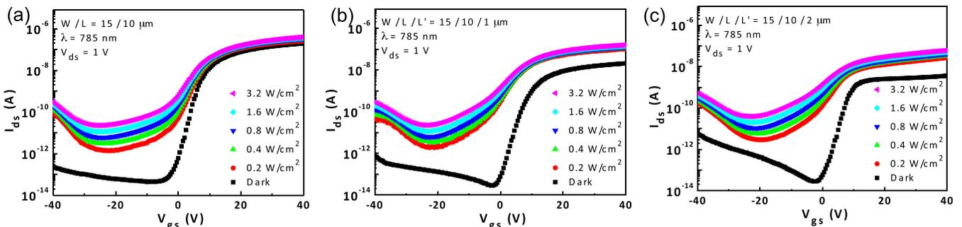
FIG. 3. Transfer curves under illumination at various incident optical power densities for  $\alpha$ -Si:H phototransistors (a) without gate underlap ( $L' = 0$   $\mu$ m), and with gate underlap of (b)  $L' = 1$   $\mu$ m and (c)  $L' = 2$   $\mu$ m at  $V_{ds} = 1$  V. Wavelength of the laser is 785 nm and incident optical power densities are 0, 0.2, 0.4, 0.8, 1.6, and 3.2 W/cm<sup>2</sup>.
