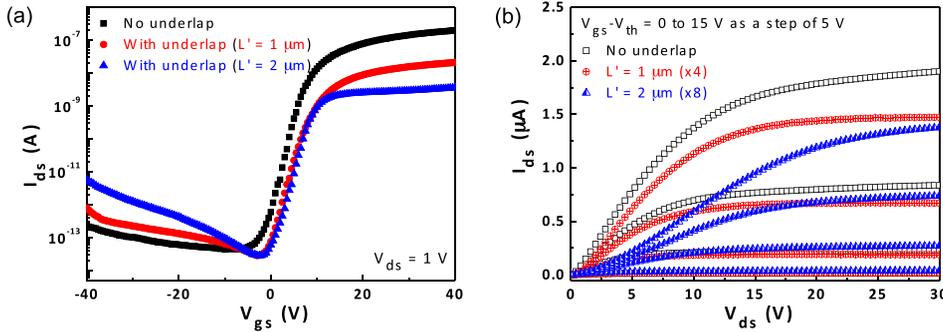
FIG. 2. (a) Transfer characteristics of the bottom-gate  $\alpha$ -Si:H TFTs at  $V_{ds} = 1$  V with various gate underlap lengths. (b) Output characteristics of the same phototransistors. The current level was adjusted for 1- $\mu$ m and 2- $\mu$ m gate underlap devices for the sake of discussion and comparison.
