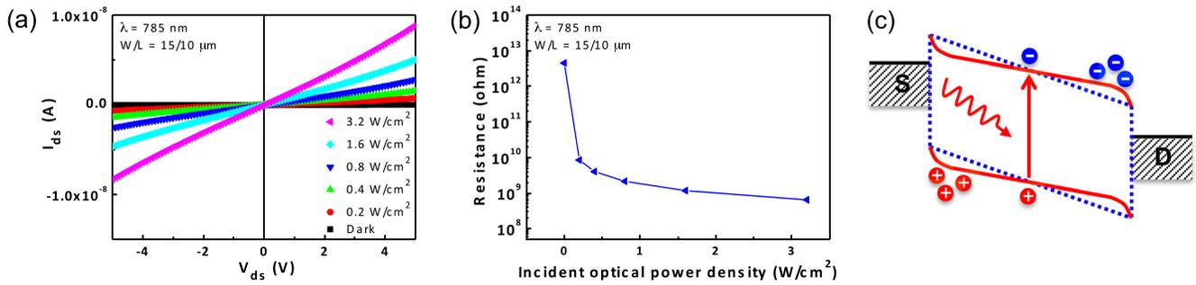
FIG. 4. (a)  $I_{ds}$ - $V_{ds}$  curves for a floating gate  $\alpha$ -Si:H TFT without gate underlap at the dark state and under illumination at various light power densities of 0.2, 0.4, 0.8, 1.6, and 3.2  $W/cm^2$  with the laser wavelength of 785 nm. (b) Resistance as a function of incident optical power density. (c) Band diagram under illumination (red solid lines) at  $V_{ds} > 0$ . Blue dotted lines show conduction and valence bands at the dark state.
