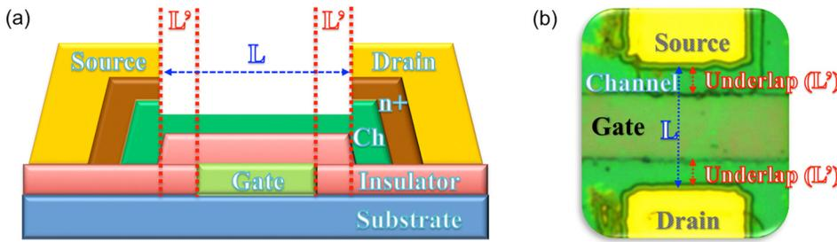
FIG. 1. (a) 2D cross-sectional schematic of a bottom-gate  $\alpha$ -Si:H TFT with gate underlap. The dashed lines indicate the length of gate underlap ( $L'$ ). (b) Optical microscope image in top view of the fabricated  $\alpha$ -Si:H TFT.
