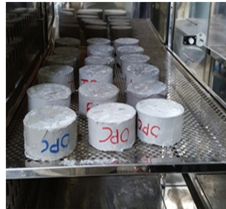
(b) Samples in the carbonation chamber
