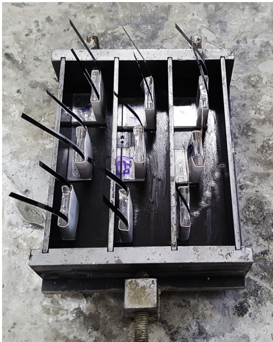
Fig. 3. Photo of mold structures of mortar specimen.
