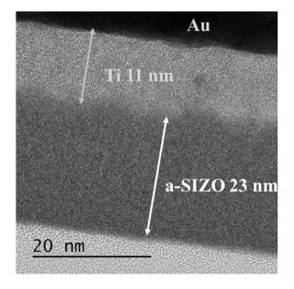
Fig. 2. Cross-sectional TEM overview of amorphous SIZO channel material.
