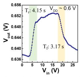
Fig. 11. Time-domain characteristics of the proposed photoinduced inverter device when exposed to red light with a power of 10.32 mW/cm<sup>2</sup>.
