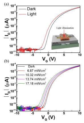
Fig. 4. Transfer curve under (a) dark/light conditions and (b) various power intensities of red illuminations.
