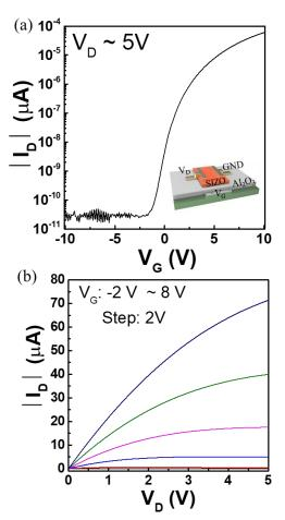
Fig. 3. Transistor characteristics in terms of (a) transfer and (b)
