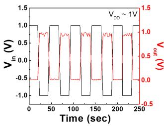
Fig. 8. Time-domain characteristics for a pulsed input voltage from -1 V to 1 V.
