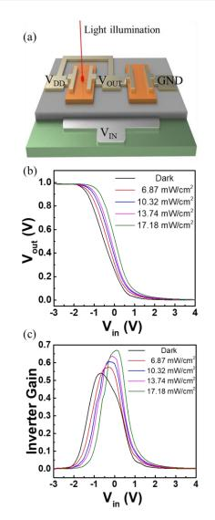
Fig. 9. (a) A schematic layout of the proposed inverter device under light illumination. (b) Inverting and (c) gain characteristics under different power intensities of red-light.
