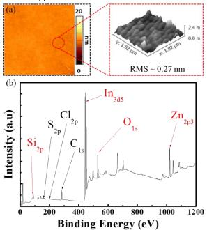
Fig. 1. (a) Surface roughness analysis of deposited a-SIZO film using the atomic force microscope (AFM) method. (b) Material characterization of a-SIZO film through x-ray photoelectron spectroscopy (XPS) analysis.
