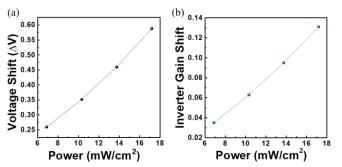
Fig. 10. The photo-responsive behavior of the proposed inverter device in terms of (a)  $\Delta V$  and (b) inverter gain shift.
