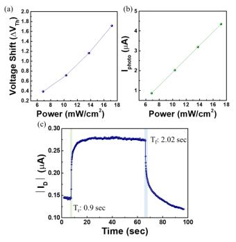
Fig. 5. The photo-responsive behavior in terms of (a)  $\Delta V_{Th}$ , (b) I<sub>photo</sub>, and (c) time-domain.
