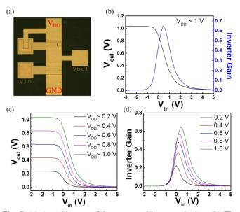
Fig. 7. (a) A real image of the proposed inverter device. (b) The inverting curve of the device with inverter gain. (c, d) Inverting and gain characteristics at different  $V_{DD}$ .
