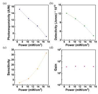
Fig. 6. The key figure of merit for photodetection parameters in terms of (a) photoresponsivity, (b) detectivity, (c) sensitivity, and (d) gain.
